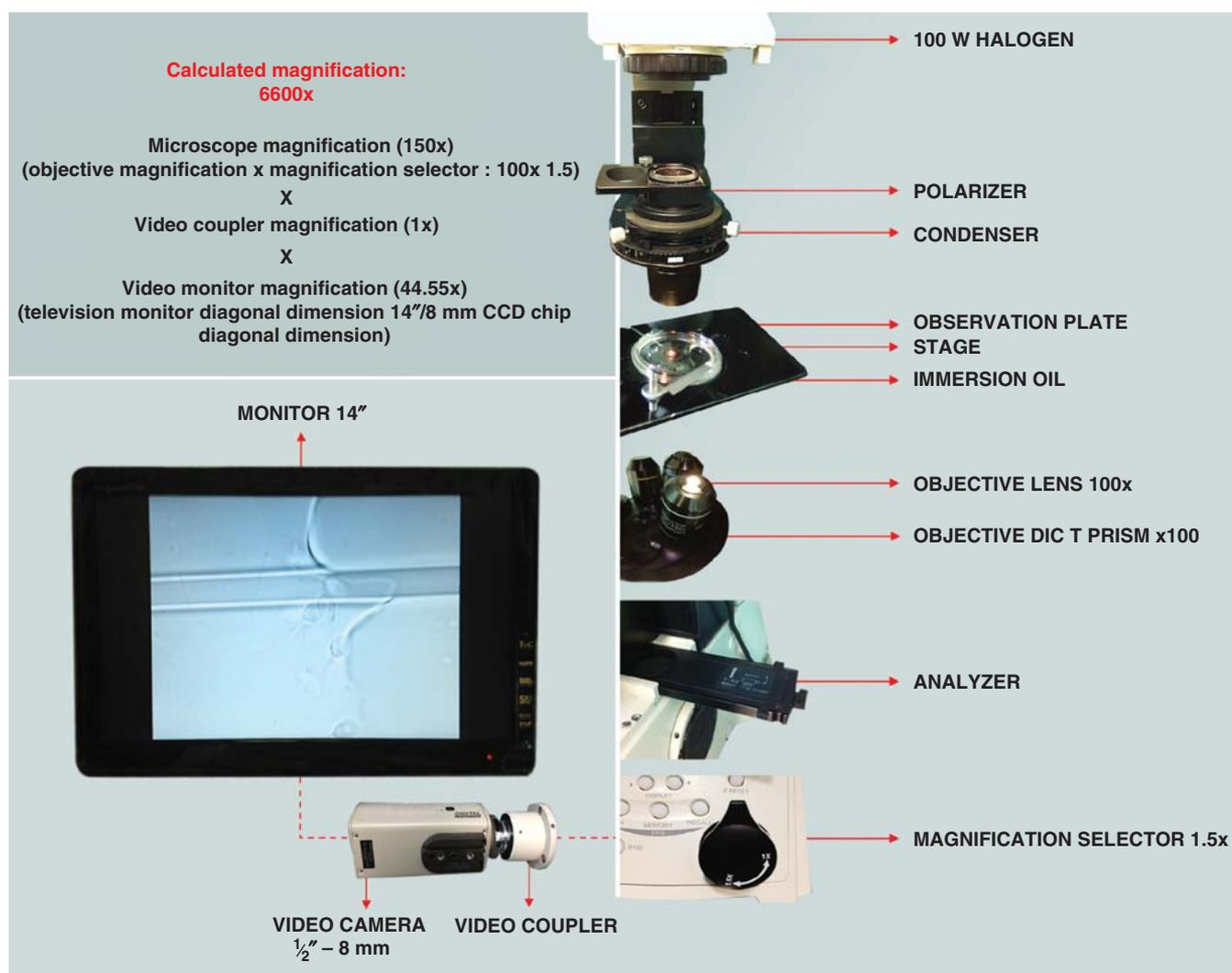
Figure 10.1 IMSI apparatus resulting in the corresponding calculated magnification. Abbreviations: DIC, differential interference contrast; CCD, charge-coupled device.
